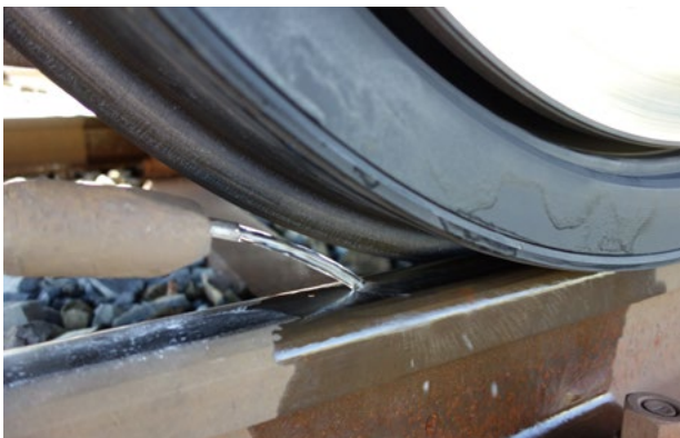
Soapy water dosing device for influencing the coefficient of adhesion
